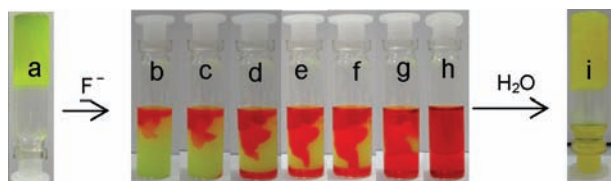
Figure 4. (a) Organogel formed from I in THF (4 mg/mL); (b) immediately after addition of TBAF (1 equiv); after (c) 1 min; (d) 3 min; (e) 5 min; (f) 7 min; (g) 9 min; (h) 10 min; and (i) after addition of 0.2 mL of water.
